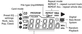
Shows radio frequency, radio preset location, folder number, CD track number, CD program location, playback time, current mode, etc.
