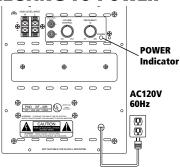
Plug the PRO-SW60P's AC power cord into an AC outlet. The POWER indicator lights red. If the subwoofer does not receive a signal for about 11 minutes, the amplifier goes into standby mode.
