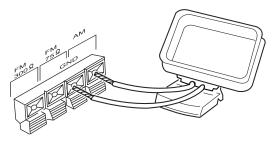
Place the antenna on a flat surface and rotate it for the best AM reception.
