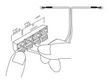
For better FM reception, you can also use a rabbit-ear TV antenna (for indoor use only) or an outdoor VHF TV antenna. To connect the TV antenna to the receiver, you need a VHF/UHF/FM splitter (not included). RadioShack stores carry a full line of quality antennas and antenna connection accessories.
