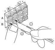
2. Press open the receiver's negative (–) black lever for the same speaker and insert the other conductor's end into the small hole. Release the lever to secure the conductor.
