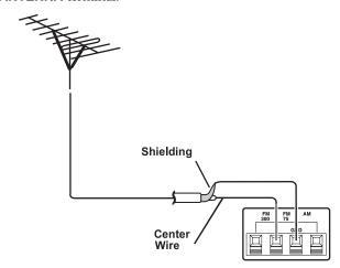
**Caution:** The cable's shielding should only touch the **GND ANTENNA** terminal.
