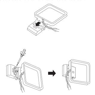
Attach the antenna wires from the AM loop antenna to the AM and **GND** (ground) ANTENNA terminals.
