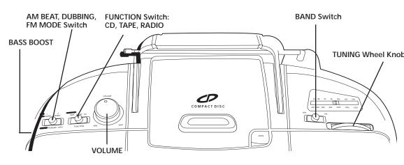
BAND Switch - Move the switch to select AM or FM
