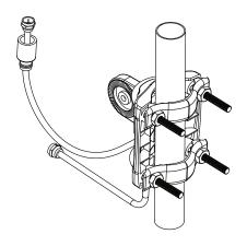
**Note:** If you used the provided coaxial cable, make sure to mount the base so that the cable exits downward.
