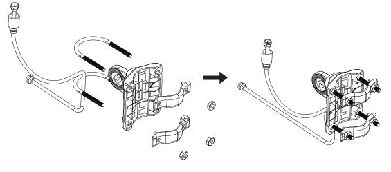
**Important:** These diagrams show the cable that came with this antenna. This cable was designed to fit under the U-bolt. If you are using a different cable, DO NOT pass it under the U-bolt as shown here. Instead, leave it outside the U-bolt and tape it to the mast.
