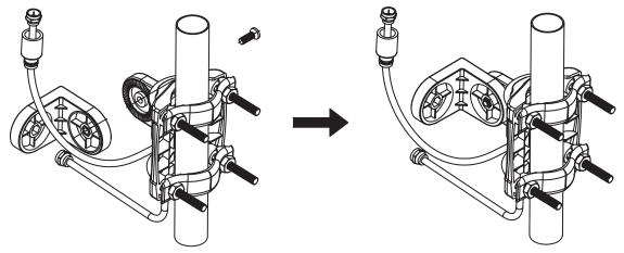
**Important:** These diagrams show the cable that came with this antenna. This cable was designed to fit under the U-bolt. If you are using a different cable, DO NOT pass it under the U-bolt as shown here. Instead, leave it outside the U-bolt and tape it to the mast.
