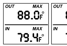
Press MEM once. The maximum (MAX) indoor and outdoor temperatures appear for about 5 seconds.
