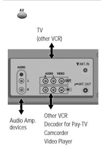
To copy to your video **from another video machine**, connect the two machines with a cable between their RCA sockets and select as programme "AV" or "F. AV" (front sockets) using the [AVI, [PR+/-], or [00] button.
