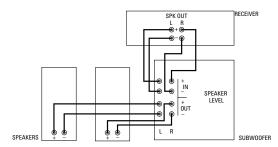
Connect speaker wires from the Receiver's front left and right speaker outputs to the subwoofer's left and right Speaker In terminals. Connect speaker wires from the subwoofer's left and right Speaker Out terminals to the left and right front speakers being used in the system.
