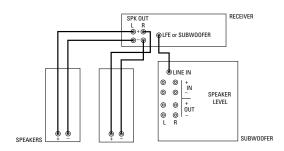
Connect an audio cable from the Subwoofer Out or LFE Out on the back of your Receiver to the Line In jack on the back of the subwoofer.
