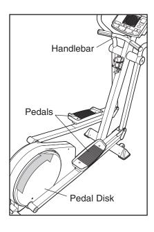
that you move the pedal disks in the direction shown by the arrow; however, for variety, you can turn the pedal disks in the opposite direction.
