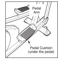
ions to the desired positions. Make sure that both pedal cushions are in the same position.
