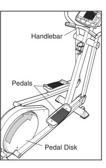
that you move the pedal disks in the direction shown by the arrow; however, for variety, you can turn the pedal disks in the opposite direction.
