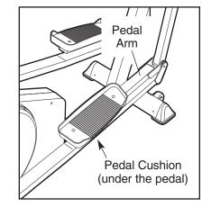
ions to the desired positions. Make sure that both pedal cushions are in the same position.
