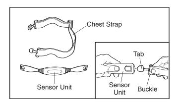
See the inset drawing above. Insert the tab on one end of the chest strap through one end of the sensor unit as shown. Then, press the end of the sensor unit under the buckle on the chest strap.
