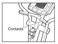
heart rate, hold the contacts; your palms must be resting on the upper contacts, and your fingers must be touching the lower contacts. **Avoid moving your hands.**  When your pulse is detected, the Heart Rate indicator above the lower display will light, one or two dashes (--) will appear in
