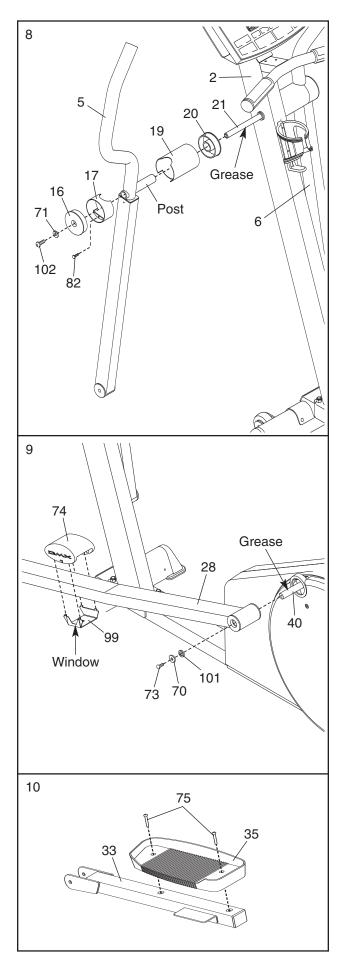
Set the Left Pedal Arm (33) on the left Pedal Cushion (74), and hold the end of the Left Pedal Arm inside of the bracket on the Left Pedal Leg (28).
