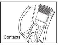
the handgrip pulse sensor, with your palms on the contacts. **Avoid moving your hands.** When your pulse is detected, one or two dashes will appear in the Heart Rate display and then your heart rate will be shown.
