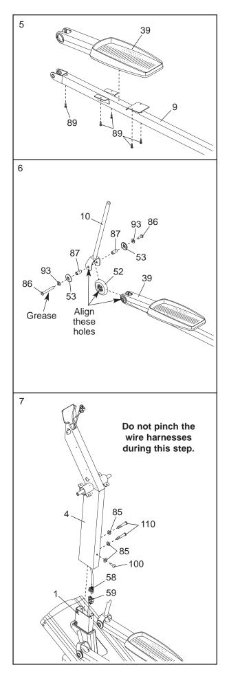
While another person holds the Pulse Sensor Bar (26) near the Upright (4), connect the upper pulse wires to the lower pulse wires. Insert the excess wire into the Upright.
