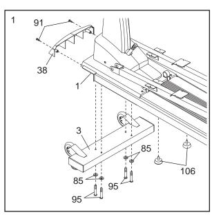
Orient the Rear Stabilizer (2) as shown. Attach the Rear Stabilizer to the Frame (1) with four M8 x 65mm Button Screws (95) and four M8 Split Washers (85).
