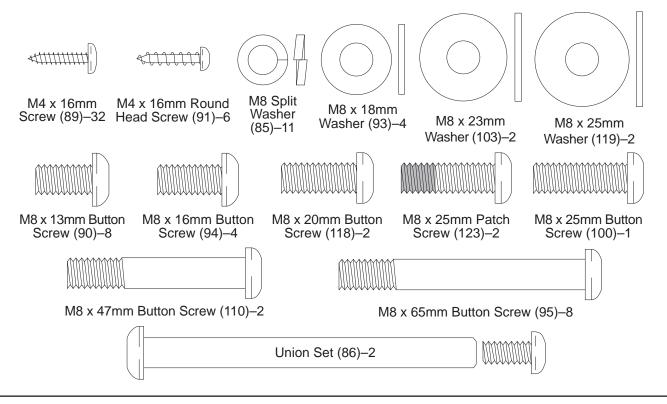
1. Orient the Front Stabilizer (3) as shown. Attach the Front Stabilizer to the Frame (1) with four M8 x 65mm Button Screws (95) and four M8 Split Washers (85).
