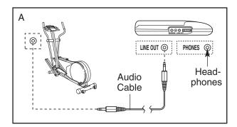
B. Plug one end of the audio cable into the jack beneath the console. Plug the other end of the cable into a 1/8" Y-adapter (available at electronics stores). Plug the Y-adapter into the PHONES jack on your CD player. Plug your headphones into the other side of the Y-adapter.
