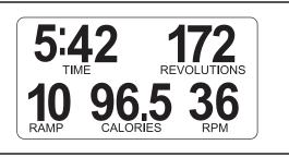
The upper right corner of the display will show the distance you have pedaled, in total revolutions. The display will also show your heart rate when you use the handgrip pulse sensor (see step 5 on page 15).
