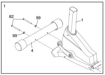
While another person lifts the Folding Frame (2), attach the Rear Stabilizer (3) to the Folding Frame with two M10 x 93mm Button Screws (82) and two M10 Curved Washers (99). Next, tighten the Center Foot (95) into the Frame (1).
