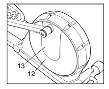
using a flat screwdriver. Next, remove the four screws (not shown) from the center of the left Disc (12). Gently rotate the Disc Cover and the Disc away from the elliptical exerciser.
