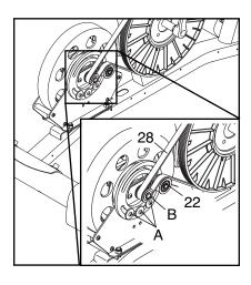
Then, tighten the three screws.
