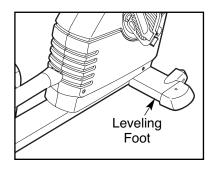
rocks slightly during use, turn one or both of the leveling feet under the front stabilizers until the rocking motion is eliminated.
