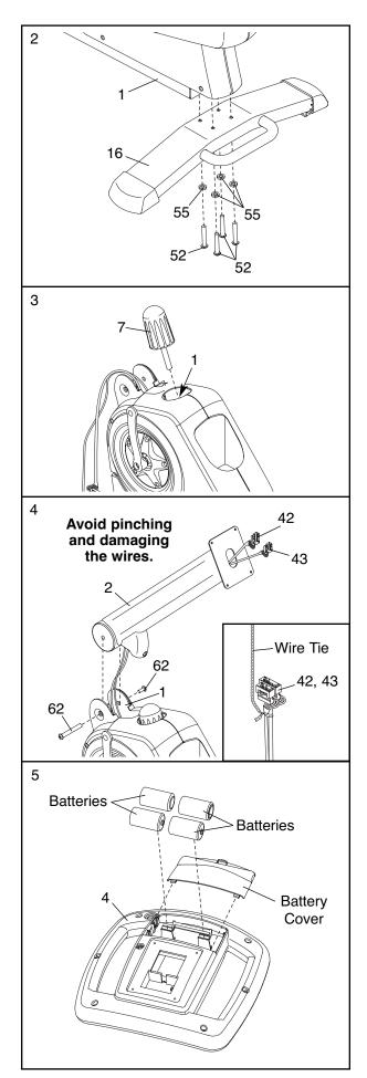
6. While another person holds the Console (4) near the Upright (2), connect the console wire harnesses to the Upper and Main Wire Harnesses (42, 43). Insert the excess wire downward into the Upright.
