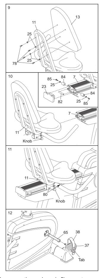
13. Make sure that all parts are properly tightened before you use the exercise cycle. Place a mat beneath the exercise cycle to protect the floor.
