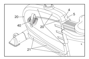
Crank Arm (not shown) so that it is pointing toward the front of the exercise cycle, and then slide off the Left Side Shield.
