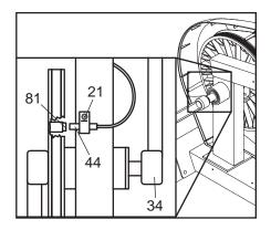
x 16mm Screw (21). Slide the Reed Switch slightly closer to or away from the Magnet. Then, retighten the Screw. Turn the Left Crank Arm for a moment. Repeat until the console displays correct feedback. When the Reed Switch is correctly adjusted, reattach the left side shield and the left pedal.
