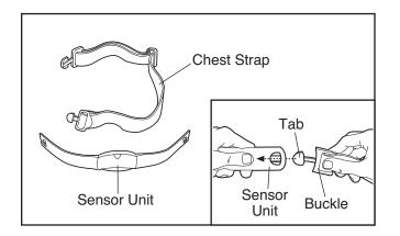
Refer to the inset drawing above. Insert the tab on one end of the chest strap through one end of the sensor unit as shown. Make sure to press the end of the sensor unit under the buckle on the chest strap. Wrap the chest pulse sensor around your chest. Attach the other end of the chest
