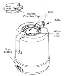
baffle, flat side down into the spout and secure with the nut. The hole on the flat side of the baffle should be facing down. It is important that you tighten the securing nut, with baffle properly in place, onto the boiling chamber before each use. Failure to properly secure the baffle and nut may result in leakage or early shut off of the AquaVié™ unit.
