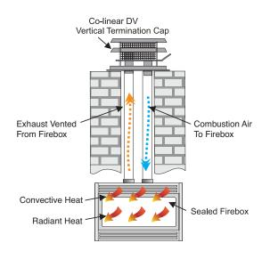
A Regency® Gas Insert is a specially engineered, sealed fireplace that slips into your existing masonry or pre-fab fireplace to create a high efficiency heating system with a beautiful fire. The airtight firebox means that you will keep all of the comforting heat generated from your Regency inside your home. Even when your fireplace is turned off, you will not lose heat up the chimney.
