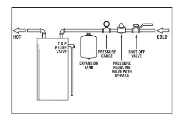
Expansion tanks are pre-charged with a 40 PSI air charge. If the inlet water pressure is higher than 40 PSI, the expansion tank's air pressure must be adjusted to match that pressure but must not be higher than 80 PSI.
