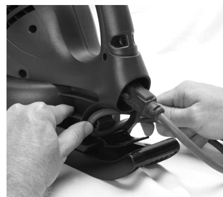
Figure 4-3: Pull extension cord loop tight around molded cord hitch
