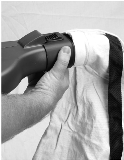
Figure 3-5: Sliding vacuum tube adapter into place
