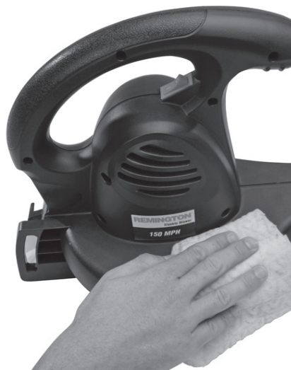
Figure 9 - Cleaning blower housing
