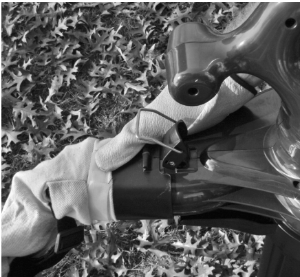
Figure 4-10: Removing bag/adapter assembly
