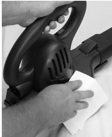
Figure 5-1: Cleaning blower/vac housing
