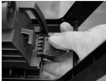
Figure 4-12: Pressing locking lever
