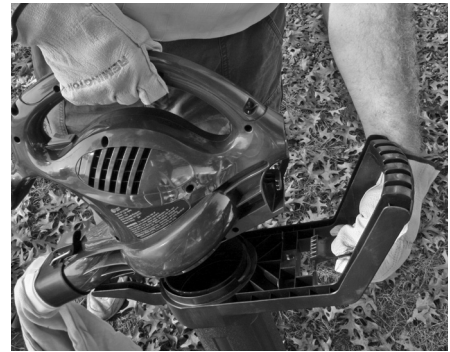
Figure 4-13: Removing vacuum tube adapter
