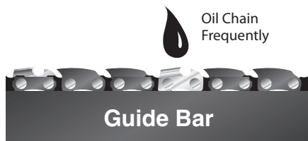
Figure 12 - Applying Oil to Chain
