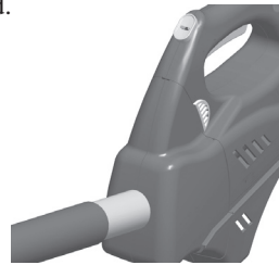
Figure 25 - Assembled Main Handle and Handle Adapter
