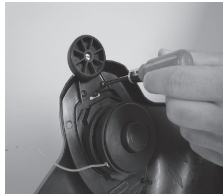
Figure 9 - Attaching edging wheel
