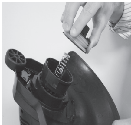
Figure 22 - Removing spool cover and spool
