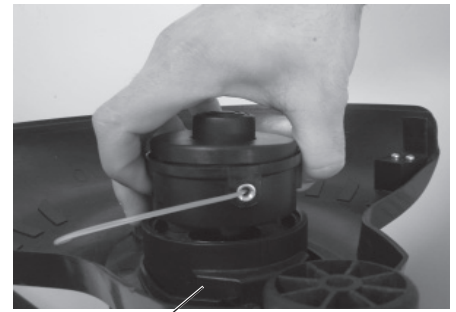
Figure 21 - Advancing trimmer/edger line
