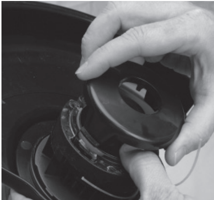
Figure 28 - Replacing spool cover onto spool housing
