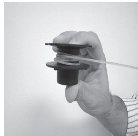
Figure 25 - Winding Line Around Spool
