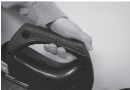
Figure 18 - Depress lockout button and squeeze trigger
