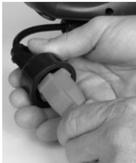
Figure 3-1: Plugging trimmer power cord into extension cord
