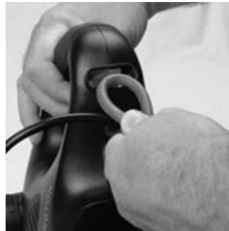
Figure 3-2: Inserting extension cord loop through bottom of handle
