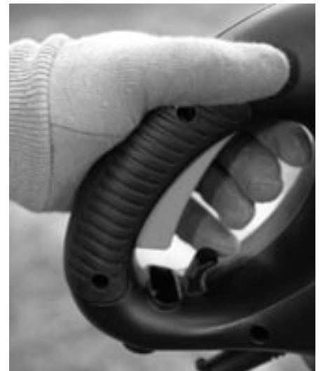
Figure 3-8: Releasing trigger switch to stop trimmer
