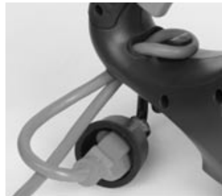
Figure 3-3: Pull extension cord loop tight around molded cord hitch
