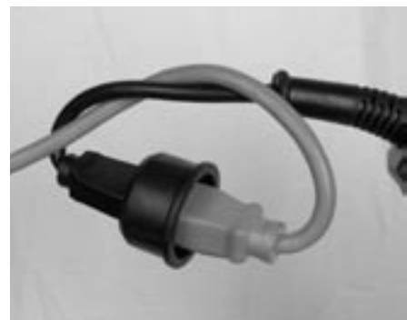
Figure 3-4: Optional method of retaining extension cord
