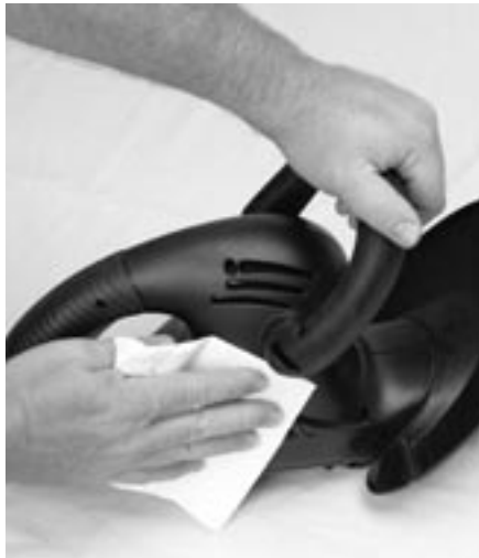
Figure 4-1: Cleaning trimmer housing
