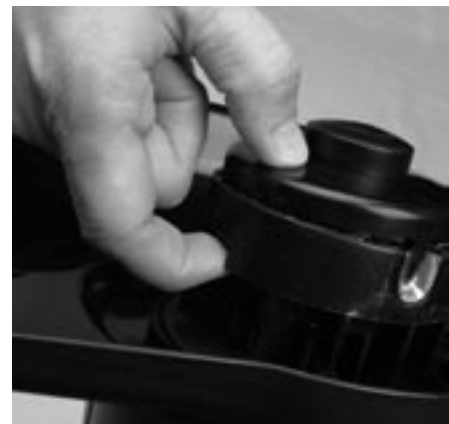
Figure 4-13: Unlocking spool cover
