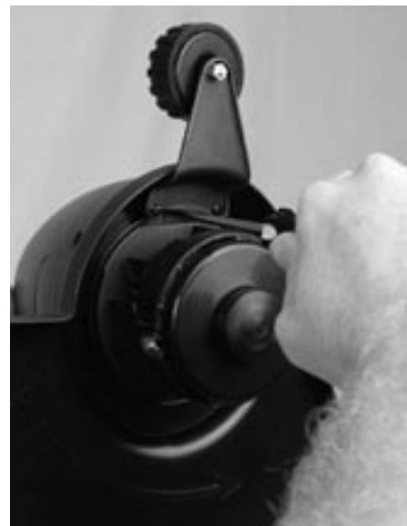
Figure 3-5: Attaching edging wheel
