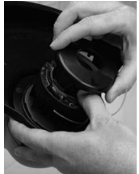
Figure 4-26: Replacing spool cover onto spool housing
