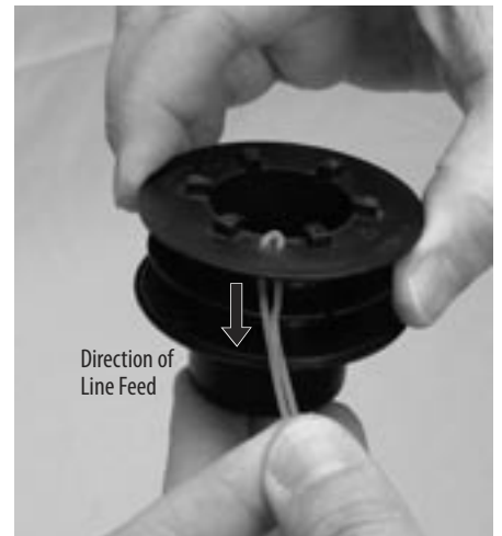
Figure 4-19: Pulling line tight
