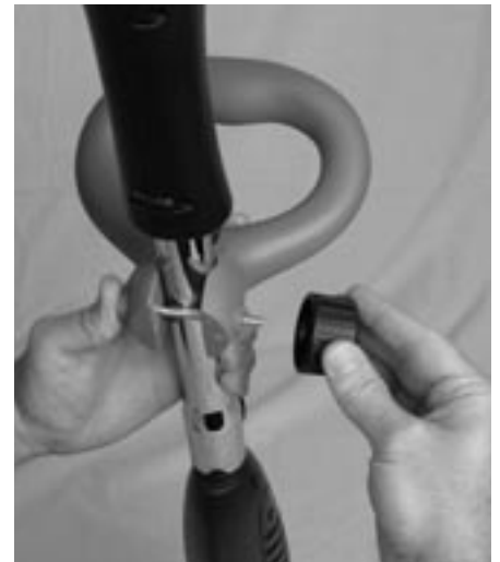
Figure 3-9: Screwing knob onto bolt
