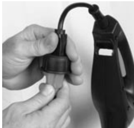
Figure 4-1: Plugging extension cord into power cord, Model ST4514B
