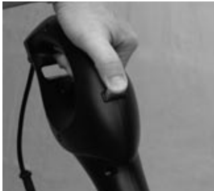
Figure 4-29: Pressing shaft rotation release button
