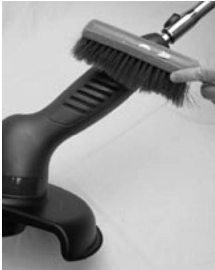
Figure 5-1: Cleaning trimmer/edger housing
