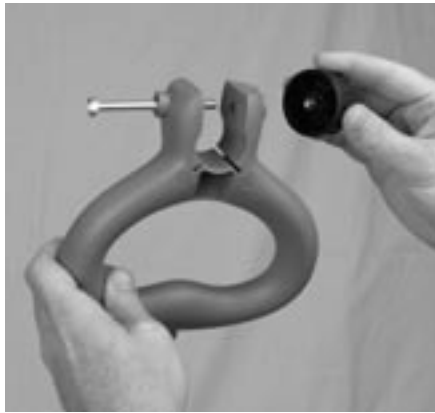
Figure 3-6: Removing knob and bolt from handle
