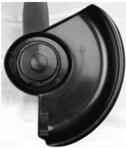
Figure 3-1: Placing cutting guard over cutting head
