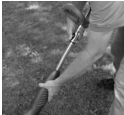
Figure 4-7: Adjusting shaft length
