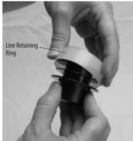
Figure 4-16: Removing line retaining ring
