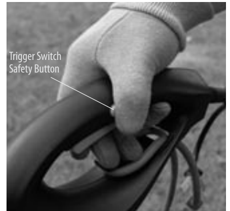
Figure 4-9: Pressing trigger switch safety button
