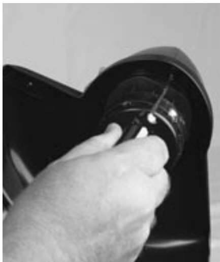
Figure 3-3: Attaching mounting screw
