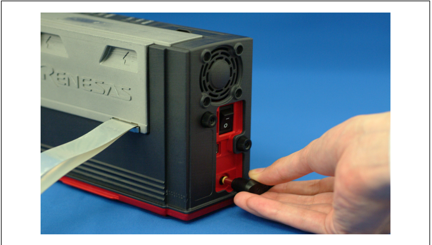
Figure 2.5 Connecting the emulator power supply
