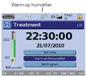
You can use the warm-up feature to pre-heat the water in the humidifier prior to starting treatment. The humidifier will be automatically detected when the device is turned on. The *Treatment* screen provides the option to start warming the humidifier. If the humidifier is heating, the related symbol is displayed at the top of the LCD screen.
