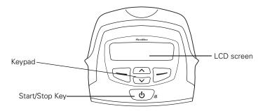
The control panel of your S8 device includes an LCD screen which displays the menus and treatment screens as well as a keypad for navigating through the menus and delivering treatment. The keypad has the following keys:
