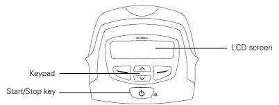
The control panel of the S8 Series II includes an LCD screen which displays the menus and treatment screens as well as a keypad for navigating through the menus and delivering treatment.
