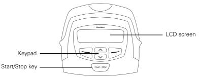
The control panel of the S8 Escape II Auto includes an LCD screen which displays the menus and treatment screens as well as a keypad for navigating through the menus and delivering treatment.
