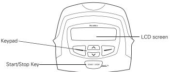
The control panel of your VPAP device includes an LCD screen which displays the menus and treatment screens as well as a keypad for navigating through the menus and delivering treatment. The keypad has the following keys:
