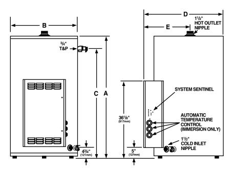
**SYSTEM SENTINEL™** – All models employ a diagnostic panel utilizing light emitting diodes (L.E.D.), corresponding to the number and location of each heating element. L.E.D.'s are energized when the electric elements are operating. An unlit L.E.D. pinpoints the exact location of a non-functioning element, making element operation diagnosis simple and positive.
