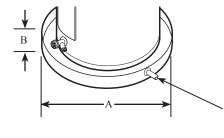
To open drain, line should be at least 3/4" ID and pitched for proper drainage.
