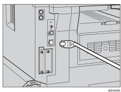
Connect the other end of the Ethernet cable to a network connection device such as a hub.
