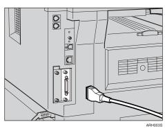
**1** Connect the other end of the cable into the interface connector on the host computer.
