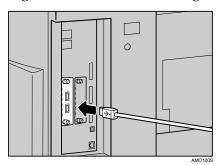
**4** Secure the USB cable using the hook.
