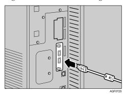
**1** Secure the USB cable using the hook.
