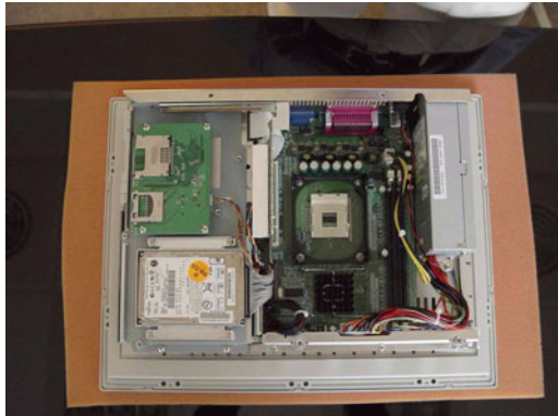
Figure 4.4: The PPC without the Rear Cover
