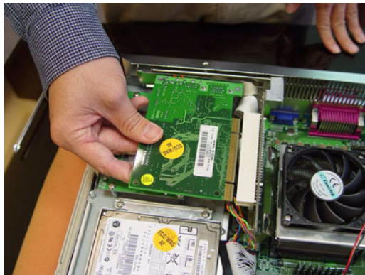
Figure 3.5: PCI bus expansion
