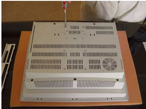
Figure 4.2: Unscrewing rear cover of the panel PC
