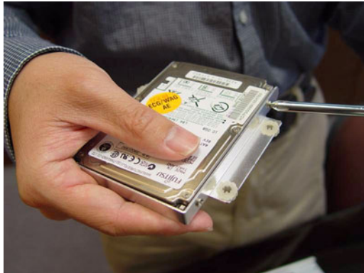
Figure 4.5: Screw the HDD metal frame to the side of the HDD
