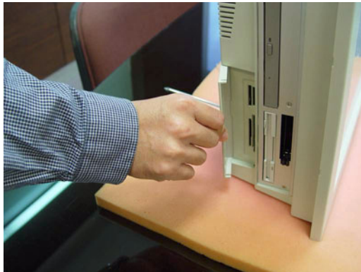
Figure 3.3: Opening the card reader's door
