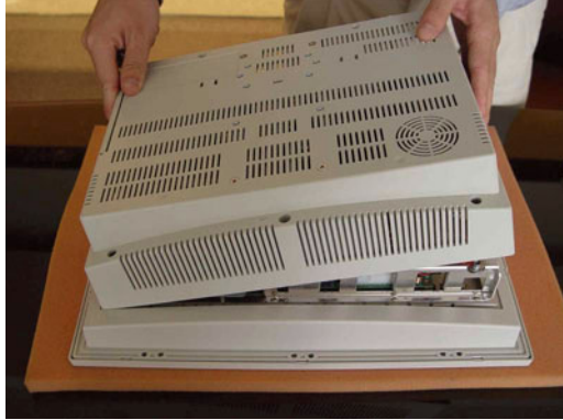
Figure 4.3: Opening the rear cover
