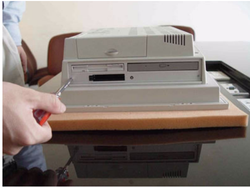
Figure 4.1: Unscrew the screw of side cover
