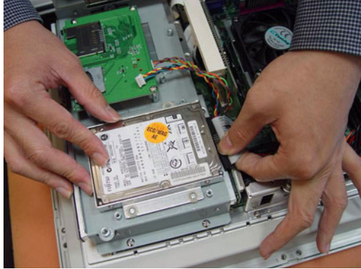
Figure 4.7: Plug the EIDE cable into the HDD
