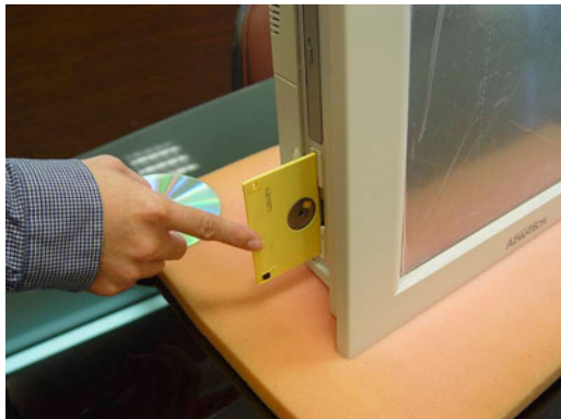
Figure 3.1: Inserting and ejecting a floppy disk
