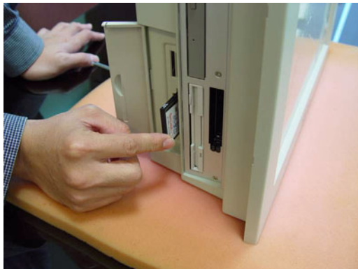
Figure 3.4: Inserting and ejecting a PCMCIA card
