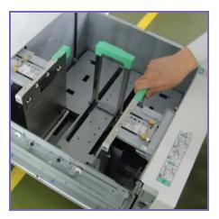
The RT5050 Large Capacity Tray can hold up to 4,000 sheets of  $13" \times 19"$  stock and can accommodate up to 300 g/m<sup>2</sup> with an Air Assist feeding mechanism to ensure reliable operation.
