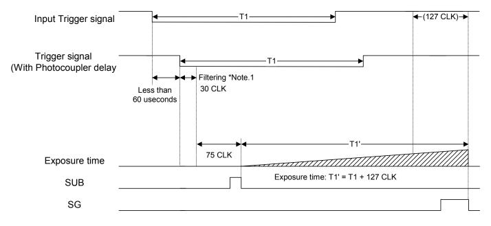
Note 1: The trigger signal will be removed by the filtering if the pulse width of the input trigger signal is less than 30 CLK. Please input a trigger signal with more than 31 CLK pulse width.
