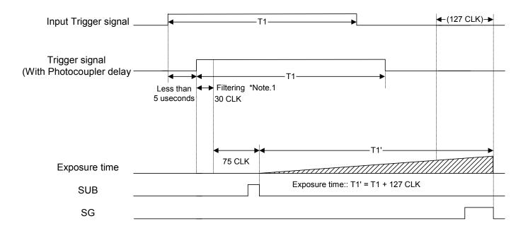
Note 1: The trigger signal will be removed by the filtering if the pulse width of the input trigger signal is less than 30 CLK. Please input a trigger signal with more than 31 CLK pulse width.
