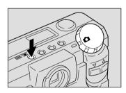
2 Decide the composition of the picture and press the RELEASE button on the remote control unit.
