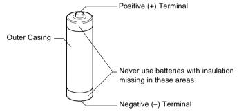
Do not use batteries with outer casings that are damaged or missing.
