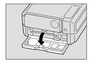
Insert the SmartMedia memory card into the card insert slot and close the card door.
