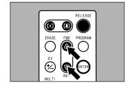
3 Select a file to be erased by pressing the FWD ( ) or REV ( ) button on the remote control unit.
