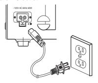
Caution: The supplied power cord has a polarized plug that fits into the outlet only one way. If the plug does not fit properly, turn it over and try again. Do not force
