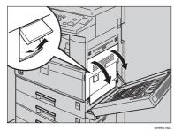
Bush down the green fusing unit's lever, as shown.
