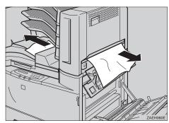
If the misfed paper is not removed in step **B**, open the upper cover of the bridge unit, and remove the misfed paper.
