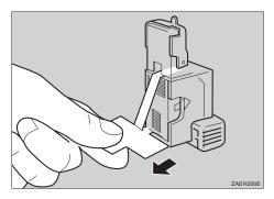
Reinstall the cartridge. It should click into place.
