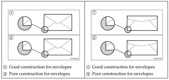
Avoid using the non-supported envelopes listed on P.38 "Paper not Supported by This Printer".
