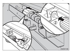
6 Check the motion of the paper feed roller to confirm that it is properly set.
