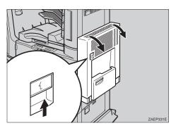
Open the right cover by lifting the catch (1), and open the upper cover of the interchange unit by pulling the handle (2).
