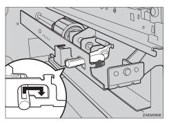
Pull the paper feed roller towards you (1), push it in a diagonally downward direction and remove it (2).
