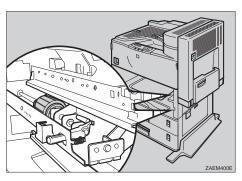
2 Raise slightly and pull the green lever that be attached the paper feed rollers inside the printer on the lower right side.
