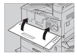
If the duplex unit is installed, close the duplex unit.
