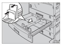
Align all four sides of the paper stack, and load it into the tray.
