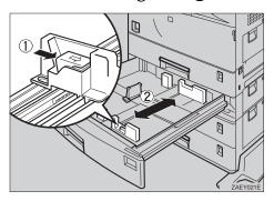
Slide the rear guide widely by pushing the releasing lever of the rear guide.
