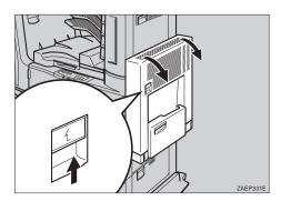
Open the right cover by lifting the catch (1), and open the upper cover of the interchange unit by pulling the handle (2).
