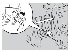
**3** Remove the empty refill case as shown in the illustration.
