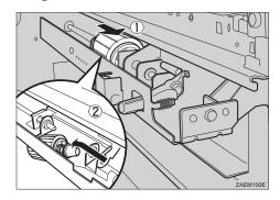
Wipe the rubber of the paper feed roller with a dry cloth.
