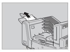
If the misfed paper is not removed in step **1**, open the right cover of the finisher.
