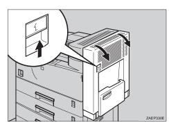
When duplex unit is installed, open the duplex unit by lifting the catch.
