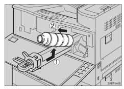
Move the new toner bottle back and forth about 5 - 6 times (①), and remove the black cap of the new toner bottle by turning it counterclockwise (②).
