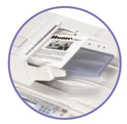
The highly reliable, single-pass document feeder is capable of scanning up to 75-images-per-minute.
