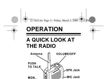
Rotate **VOLUME/OFF** to turn the radio on and off and adjust the volume.
